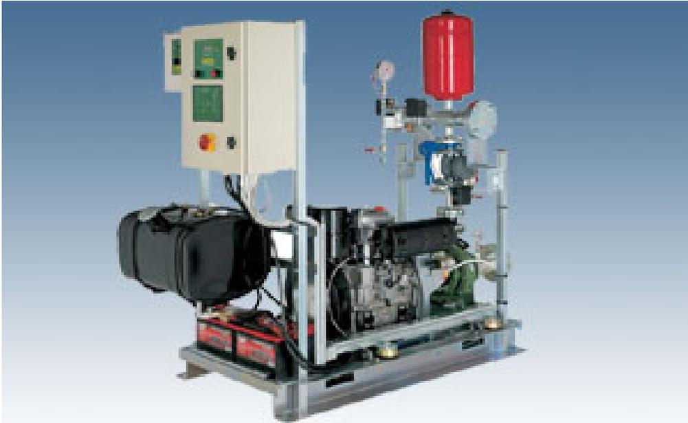
EN 12845 compliant booster units for automatic fire-fighting systems. The standard version comprises a diesel pump that can be coupled with one standardised electric pump, together with a compensation pump, if required.
